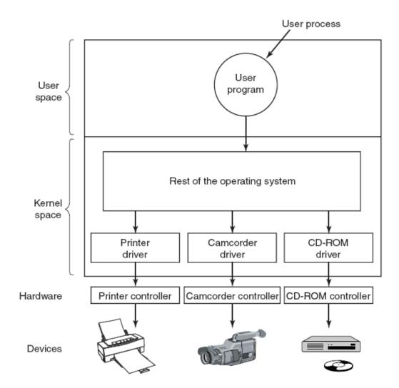
Logical positioning of device drivers. In reality all communication between drivers and device controllers goes over the bus.
