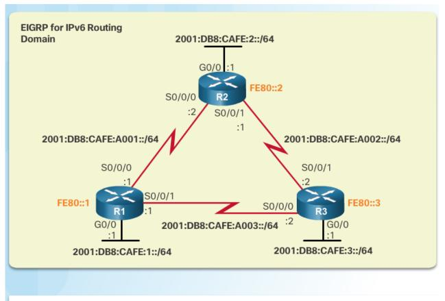
The FE80 address represents the link-local address assigned to each router.
